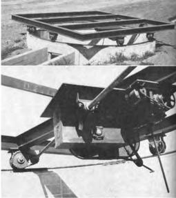
the photo. The heavy steel frame is welded to the wheel bearings, and carries the phytotron unit.
