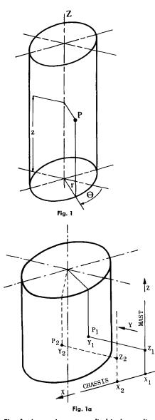
Fig. 1. Any point on a cylindrical coordinate system can be defined by three variables:  $r, \Theta$ , and Z. Fig. 1a. Relationship of cylindrical coordinate system to movements of mast, chassis, and boom as used in a man-positioner for picking fruit.
