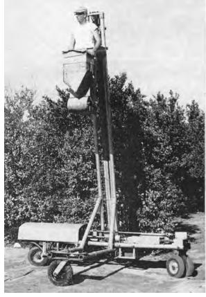
Principles of cylindrical coordinate system were used at Riverside in development of research prototype of commercial power ladder now in production.
