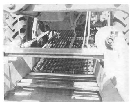
Close-up front view of 1965 harvester showing blade, the four pickup rolls, and the channel-type separating conveyor.
