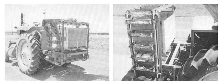
Cross conveyor and collection bin. For hand sorting, basket dumping guides at top center, left photo, are replaced with straight guides that keep baskets upright all the way across top leg. Side view, right photo, showing relation of cross conveyor to discharge end of separating conveyor. Plywood deck that usually rests on frame in front of bin was removed for photograph.
