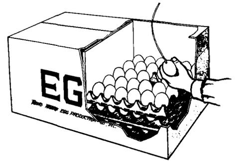
Egg with thermocouple wire for temperature measurement was placed near center of each case during the test procedure.
