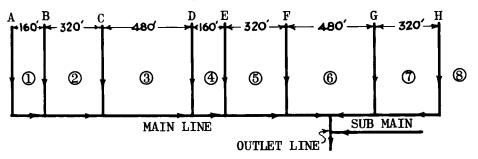
Stations (1), (2), and (3) in line layout sketch above were recorder wells. Stations (4) through (8) were observation wells only. Line details are specified in table below.
