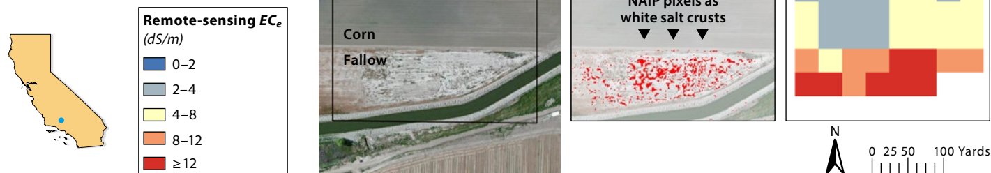
Fig. 4. Example of inaccuracy of remote-sensing estimations in a heterogeneous field with lower salinity values: (A) National Aerial Imagery Program imagery at a test site in Stratford (Kings County) on July 8, 2003; (B) ground-truth root zone (0 to 4 feet) salinity measured by Scudiero et al. (2014) through apparent electrical conductivity ( EC_a ) measurements and soil sampling; and (C) remote-sensing salinity estimations.
