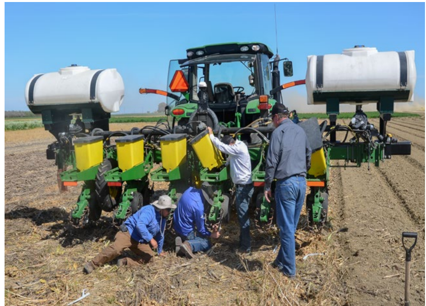
Research colleagues from California Ag Solutions, Madera, Calif., assist with John Deere 1730 no-tillage planter adjustments for garbanzo seeding. Photo: Jeffrey P. Mitchell.
