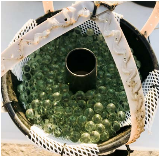
A dirty dust collector used by researchers to monitor air quality. Photo: Mark Swenson.
