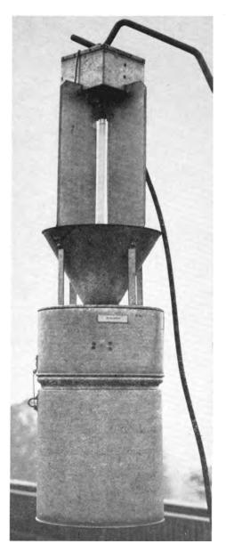
Blacklight insect trap with omnidirectionalpositioned 6-watt lamp.
