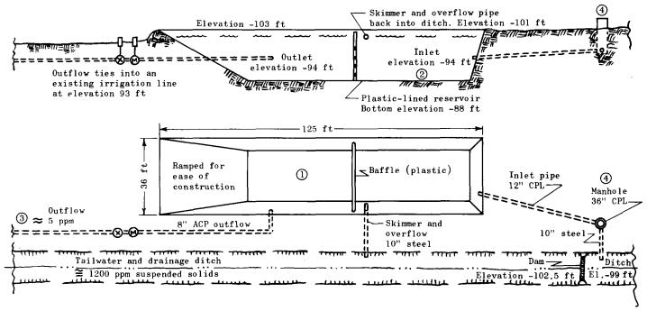
1. Reservoir large enough to give the retention time required for settling the suspended solids. 2. Reservoir settling area below inlet and outlet pipes is large enough to require cleaning once a year and still not require cleaning close to the plastic. 3. Discharge ties into an existing gravity irrigation main for reuse. 4. Manhole on inlet pipe to permit cleaning pipes if required.
