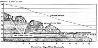
Graph 4. Depth of water table below ground surface on John Jones plot, Mecca. Graph shows average of 44 auger holes uniformly distributed throughout the 23.5 acre area. Each hole was located 12 ft away from an old tile line, already in place when the trial was begun. Four pea gravel lines (R, S, T & U) were installed in March 1966, one (V) was installed in Feb. 1967.
