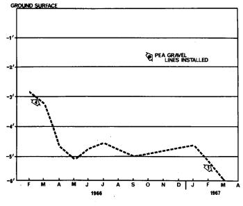
Graph 3. Profile of John Jones orchard, Mecca, Oct. 28, 1966, during irrigation (same an methods and notation as in graph 1). New pea gravel lines were carrying most of the water, had no water over them, and had lowered the general water table. (Water flow calculations were made by G. J. Hoffman, U.S. Salinity Laboratory, Riverside.)
