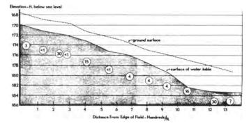
Graph 1. Profile of John Jones orchard, Mecca, Feb. 1966 before installation of new tile drains. Circles represent tile drains with top of circle at elevation of the top of the pipe. Figures in circles show flow from end of lateral in gpm/1000 ft of pipe. Water table determined from piezometers set on top of drain in the gravel envelope. Grove had not been irrigated for two months.
