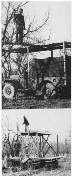
Two-stage pruning platform for pears with slipboards on upper deck. Compressor is mounted on tractor.
