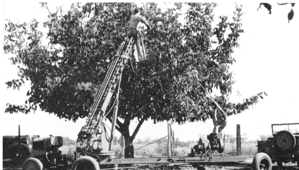
Pneumatic knockers, or limb-shakers, in the hands of skilled operators speed up mechanized harvesting.
