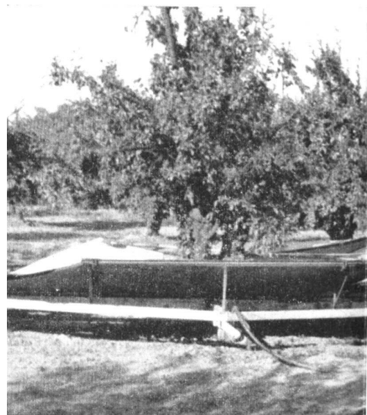
Newly designed prune catcher is pushed by tractor onto conveyor belts to be carried to storage
