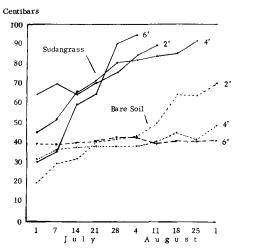
GRAPH 1. AVERAGE TENSIOMETER READINGS AT THREE DEPTHS COMPARING BARE SOIL WITH SUDAN-GRASS PLANTING.
