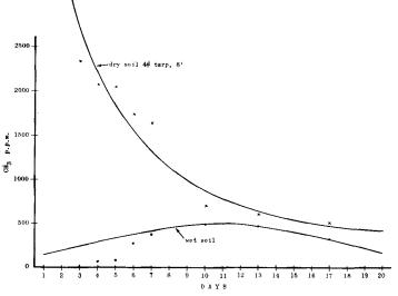
GRAPH 2. COMPARSION OF WET AND DRY SOIL IN THE PENETRATION OF METHYL BROMIDE (4 POUNDS PER 100 SQUARE FEET), AS MEASURED DOWN TO 8 FT DEPTH.
