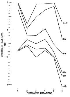
Hydraulic head loss in the gravel of the stream channel where no surface sediments were present. The numbers at the right denote the depths of the piezometers.
