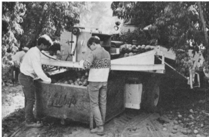
Single-unit machine, left photo, extends catching frame around tree hydraulically, and fruit is brought to rear on each side. Shaker half of two-unit machine, right photo, shown in position and shaking fruit.
