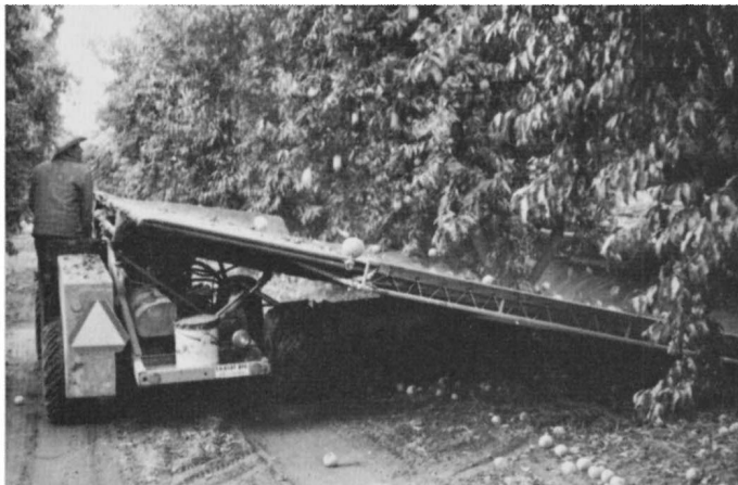
Single-unit machine, left photo, extends catching frame around tree hydraulically, and fruit is brought to rear on each side. Shaker half of two-unit machine, right photo, shown in position and shaking fruit.
