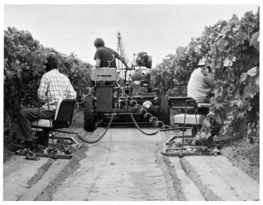
Experimental unit for towing cane cutting sleds and providing power for pneumatic shears in vineyard tests for mechanical harvesting of raisin grapes.
