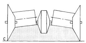
Rolling cone press with top press cylinder for closing a reshaping experimental 60-inch bed with midbed furra after planting.
