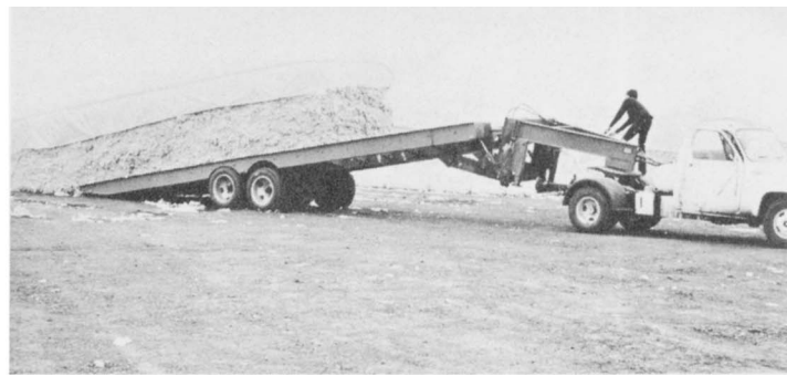
A van-type trailer (left photo) in position for loading a module. A hydraulic-powered winch pulls the module into the van. Front and rear van openings are covered with canvas for transport. Right photo shows loading of a 32-ft module at the gin yard, preparatory to ginning. This type of open trailer shown pulled by a one-ton truck, is intended primarily for highway use. Gin-yard trailers are similar, but with straight tongues and no brakes or lights, and are usually pulled with farm tractors.
