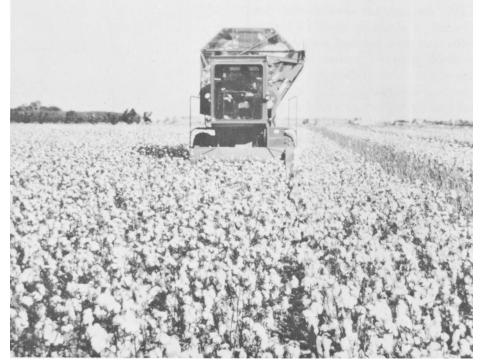
Field of narrow-row cotton at the West Side Field Station being harvested with finger stripper harvester. Lint yield from this field was over 2½ bales/acre.
