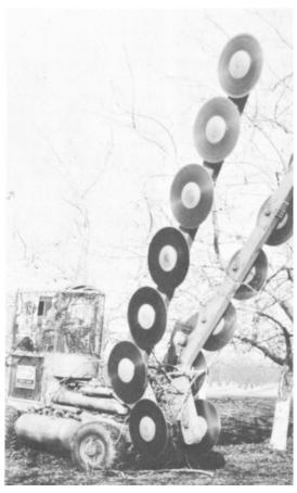
Walnut hedging machine used in these Tulare County trial featured seven circular saw blades mounted vertically on two booms, allowing trimming from either side of the row withou turning around.
