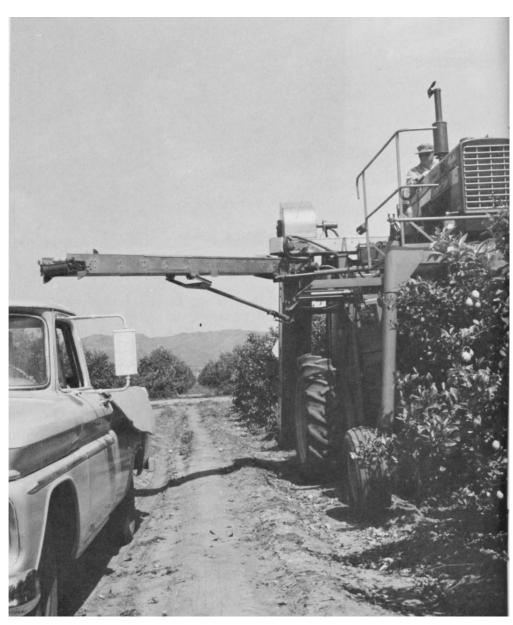
Fig. 1. Chisholm-Ryder grape harvester removing lemons from close-set trees near Santa Paula. Fruit is conveyed into cushioned bed of pickup truck. Closeset row of young lemons was previously mechanically hedged and topped.
