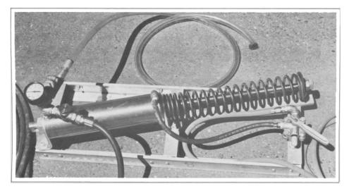
Cylinder, valves, and pressure gauge of injection machine.
