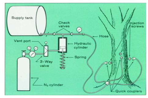
Essential parts for pressure-injection machine. Fittings necessary to connect parts are not shown; fittings vary, depending on brand or size of the components.
