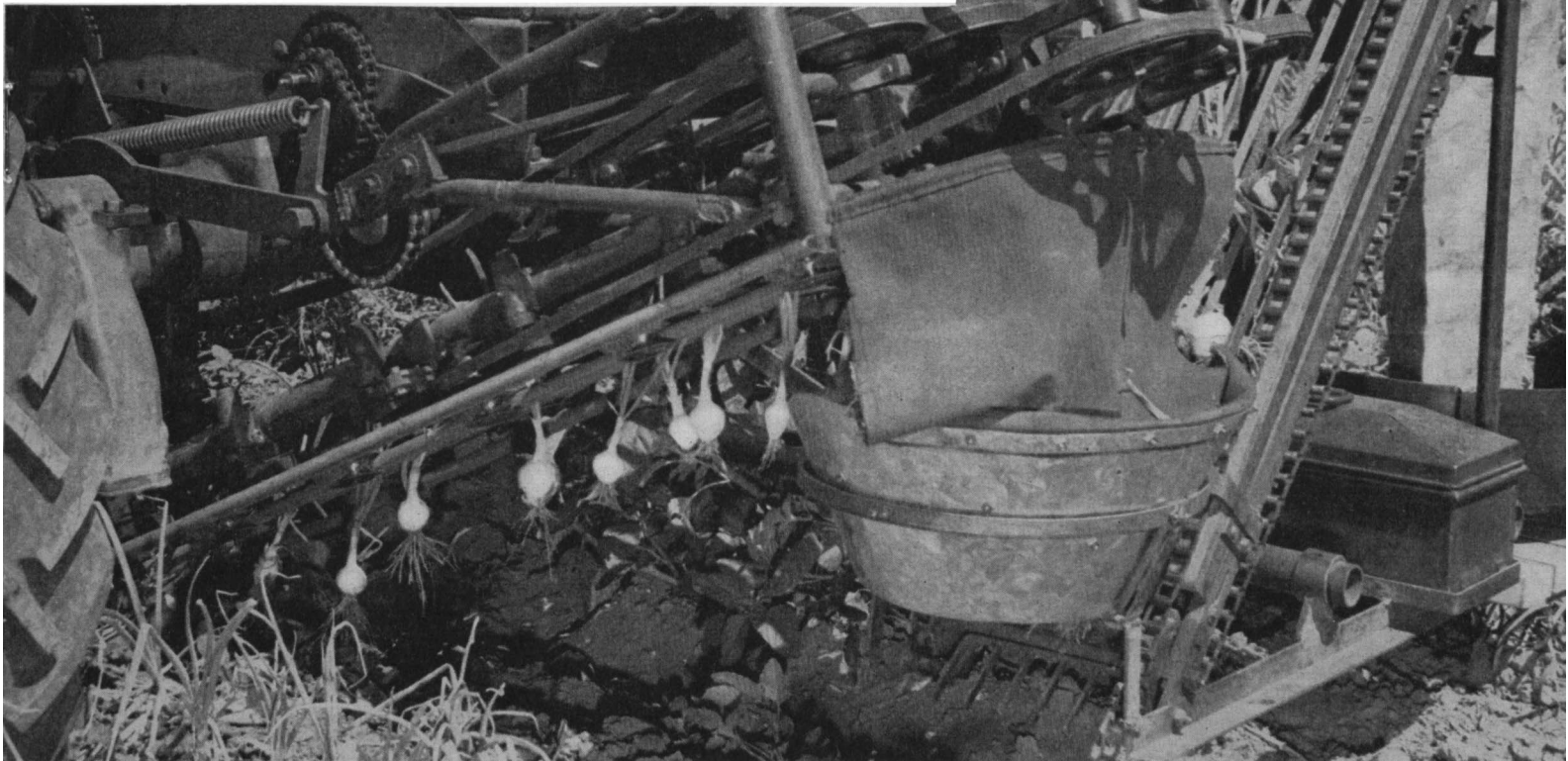
Mechanical harvester in operation on bed planted onions. After topping, onions are pulled, carried up along conveyor belt and dropped into a sack.
