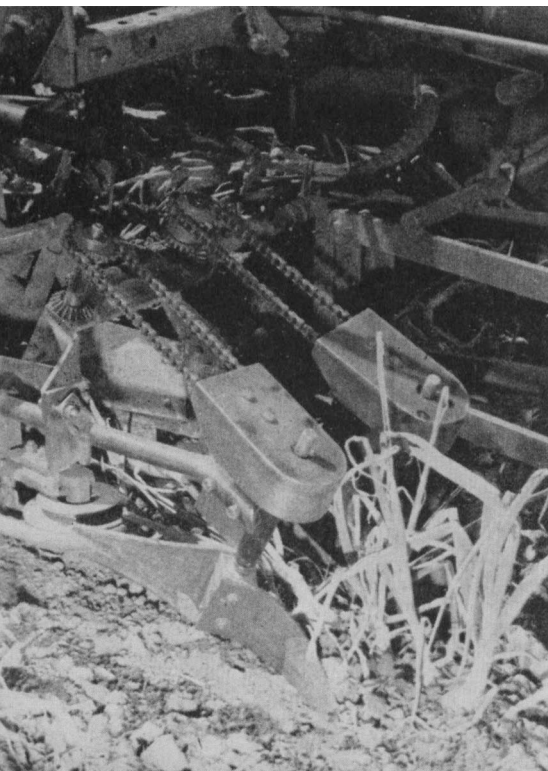
Knife blade of harvester, adjustable as to depth and angle of cut, frees onion bulbs from roots.
