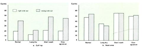
Fig. 2. Effect of laundry treatment on number of cycles until minor damage occurred on cotton durable-press cuffs (the fewer the cycles, the greater the abrasion).
