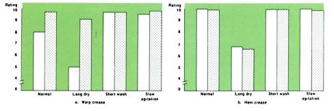
Fig. 3. Effect of laundry treatment on edge abrasion rating of cotton durable-press cuffs (the lower the rating, the greater the abrasion).
