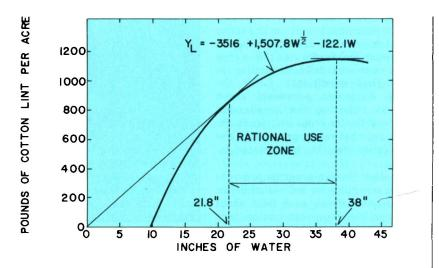
Fig. 3. Yield-water function for cotton, with the minimum and maximum water amounts that should be considered in a production system.
