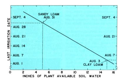
Fig. 2. Relation between soil-water-retention capability and last intgation date to achieve 98 percent of maximum yield.
