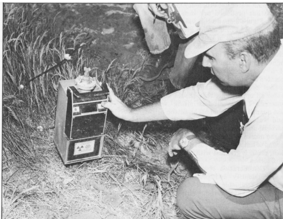
Dr. Melvin Campbell of the US Bureau of Reclamation operates the lightweight neutron probe instrument that he helped to design. The probe is placed over metal tubing, which has been installed permanently in the ground, and counts hydrogen ions in the soil near the tube. This ion count is directly related to the quantity of water in the soil and available to the plants. The instrument is calibrated for each field separately.
