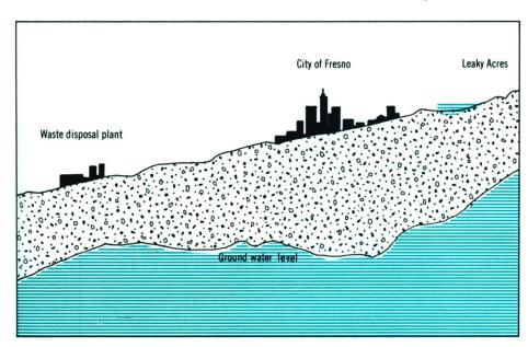
Schematic diagram of the land and water table from the city's ground-water recharge basin (Leaky Acres) to the waste disposal plant.
