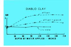
Fig. 2. SAR values of saturation extracts of Diablo clay (O- to 3-inch depth) versus total depth of water applied.
