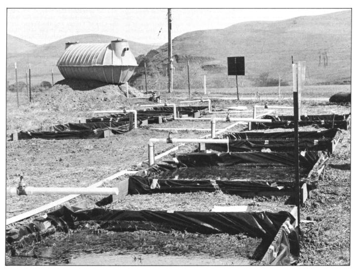
View of water percolation basins on Diablo clay soil. Fibergiass septic tank in background served as storage tank for effiuent water.
