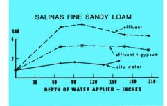
Fig. 1. Sodium adsorption ratio (SAR) values of saturation extracts of Salinas fine sandy loam (O- to 3-inch depth) versus total depth of water applied.
