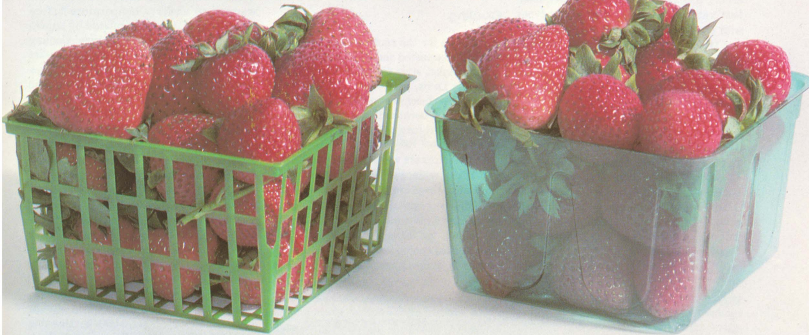
Fig. 1. Tests compared baskets of open-mesh extruded plastic (left) and solid-sided moulded plastic (right).
