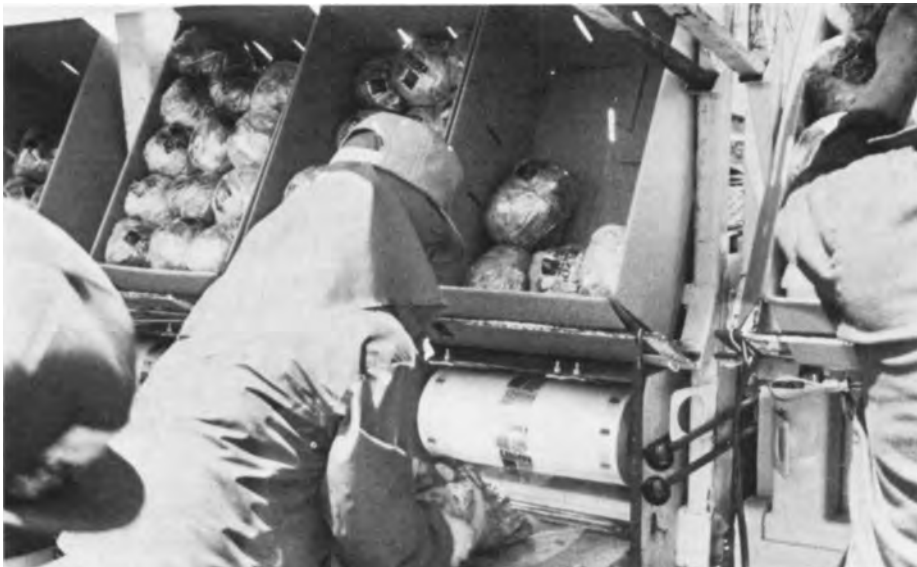
Workers are shown film-wrapping and packing head lettuce on a harvesting machine. Wrapped lettuce accounts for a significant portion (about 15 percent) of California's lettuce production. University research has shown the need for careful selection of the type and method of wrapping to allow adequate cooling of the packed lettuce.
