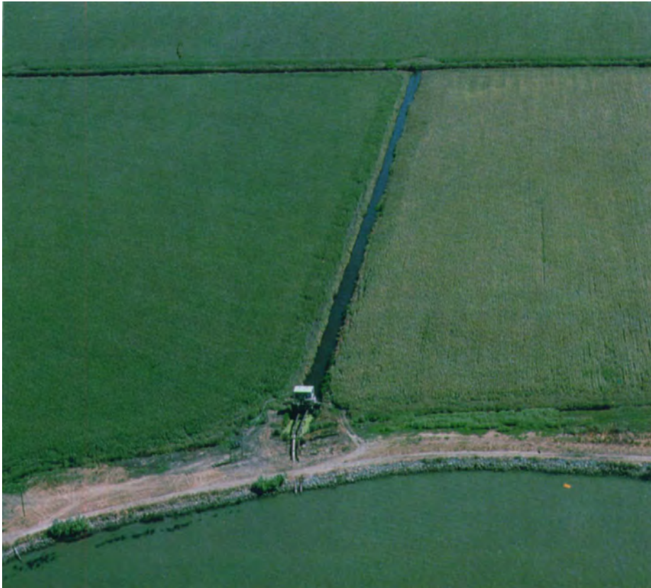
Delta farmlands are crisscrossed with drainage ditches. Here, a main drain leads to the levee where a pumping station lifts water back into the channel.
