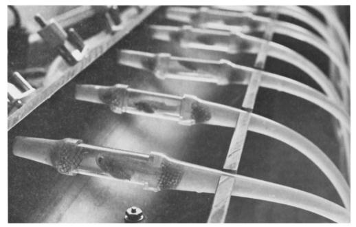
Multiple-chambered, flow-through respirometer measures metabolism of mosquito fish under various conditions.
