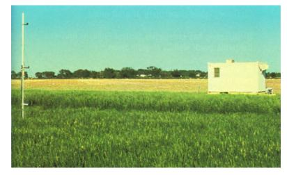
Field laboratory and temperature mast in rice paddy at U. C., Davis, automatically record rice canopy temperatures.
