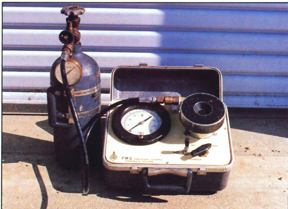
Portable pressure chamber for measuring leaf water potential is small enough to be hand-carried to measurement site.
