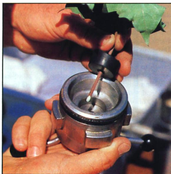
Leaf and intact petiole are inserted into underside of chamber lid and subjected to negative pressure.
