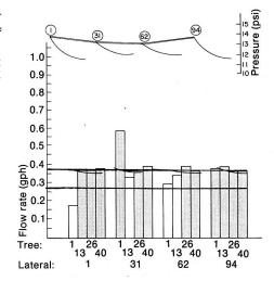
Fig. 5. When emitter plugging is a problem, lowest quarter of discharges tends to be randomly distributed.
