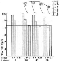
Fig. 4. Lowest quarter of discharges at ends of driplines indicates excessive pressure loss in driplines.
