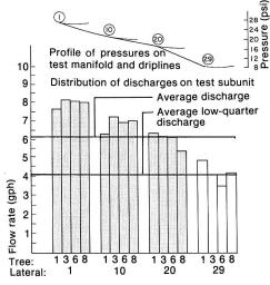
Fig. 3. Lowest quarter of discharges (nonshaded) in last dripline characterizes pressure loss within manifold.
