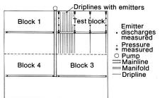
Fig. 1. Typical trickle system.
