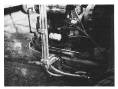
Close-up of attachment of vertical boom on conventional horizontal-boom weed sprayer. Bolts and brackets permit easy removal
