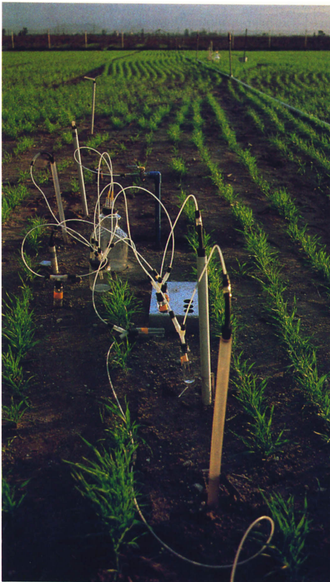
Monitoring stations consisting of tensiometers, salinity sensors, and neutron probes measured chemical and water status at 16 locations in a 3.5-acre field irrigated with blowdown water.
