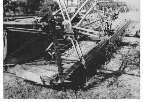
Close-up view of a windrow-swather. The vertical cutter in the foreground separates the cut material from the standing growth. The pick-up reel contributes to a cleaner job of cutting and lays the material back onto the canvas draper which conveys it to the left side of the swather.
