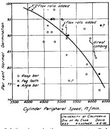
Relation of germination percentage to cylinder speed, for various types of combines. No significant differences are evident between the three types of cylinder. Seed moisture contents ranged from 5.2% to 7.5%.
