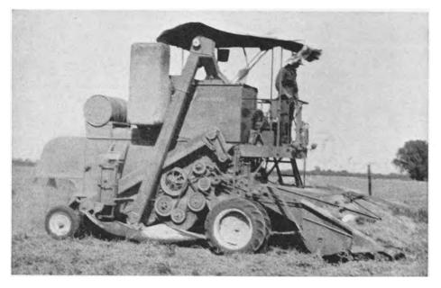
Self-propelled combine harvesting in a field with heavier-than-average windrows. The canvas sheet suspended beneath the machine catches any seed that leaks out. The ground-driven belt-type windrow pick-up was the most satisfactory type observed. The windrow here is being lifted with a minimum of disturbance.
