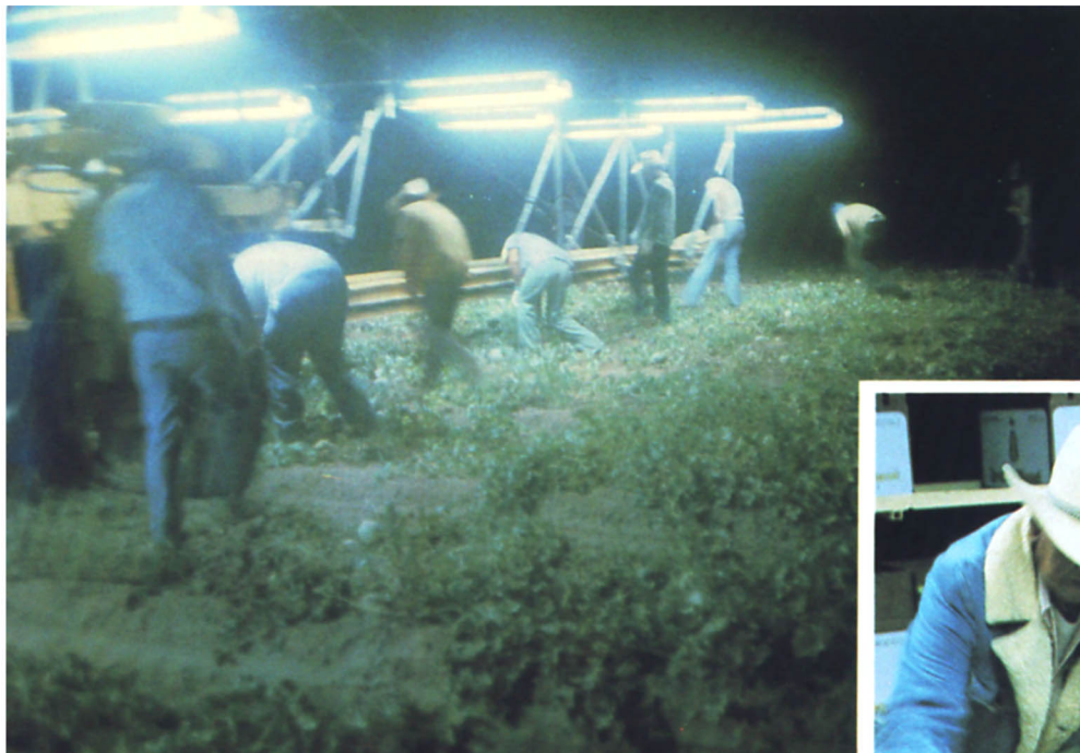
Fluorescent lamps mounted on harvesters provide the uniformity, brightness, color balance, and overall visibility to harvest melons (left), broccoli (below), and other crops during the cool nighttime hours.
