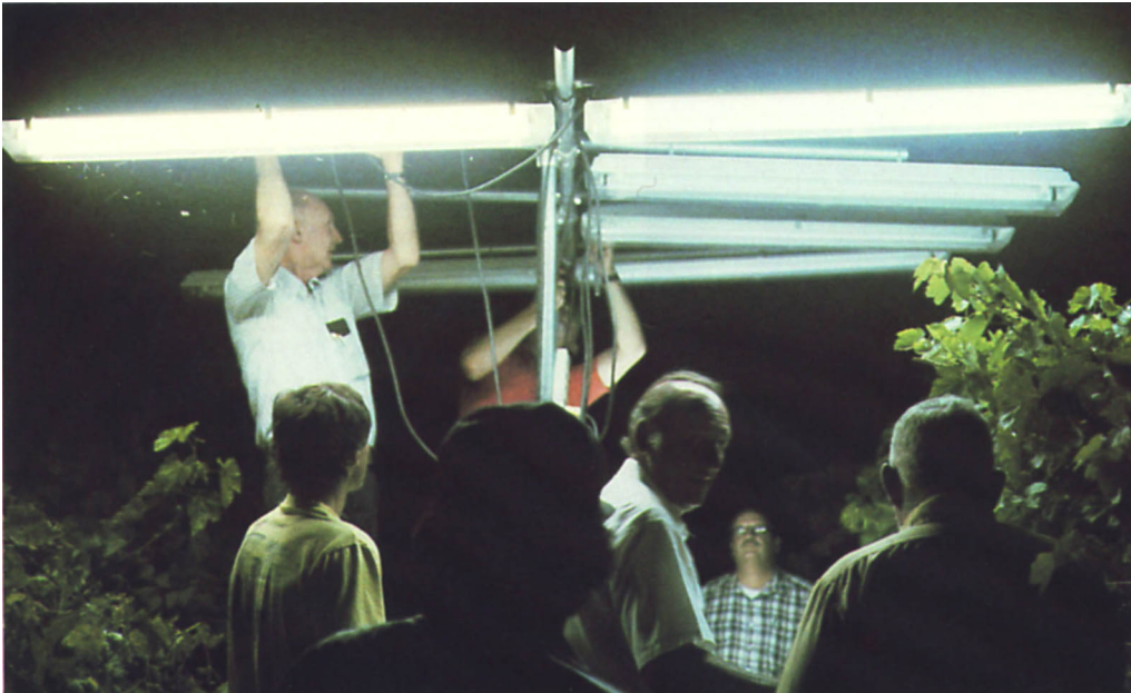
UC agricultural engineers worked with industrial lighting specialists to develop a fluorescent lighting system that could be installed on harvesters and make possible nighttime picking of perishable crops in hot southern California desert valleys.
