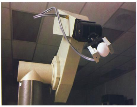
A more advanced state-of-the-art Puma 560 robotic arm markedly speeded up the egg candling process over the prototype model. The goal is to develop an intermediate model that is faster than the Rhino but less costly than the Puma.
