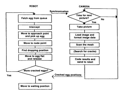
Fig. 1. Candling system block diagram.
