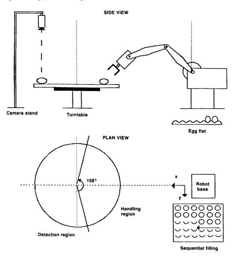
Fig. 2. Laboratory model physical layout.
