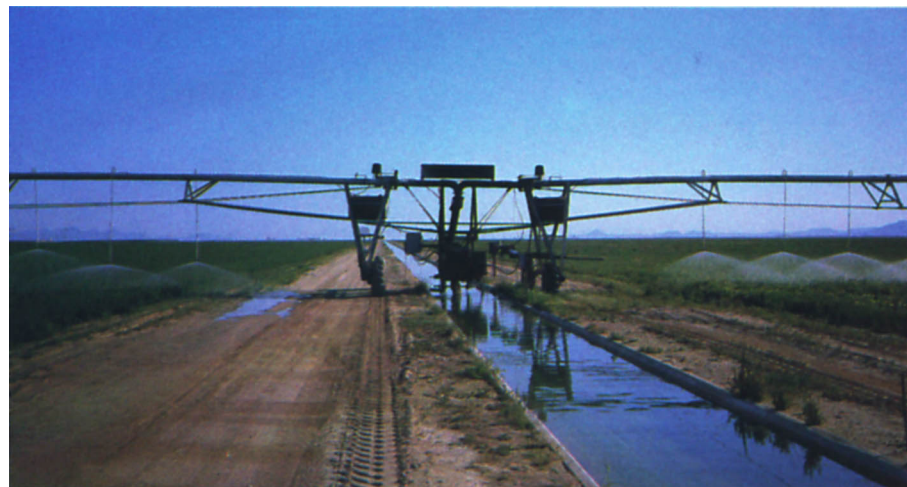
Continuous- or linear-move sprinkler systems are generally believed to have higher distribution uniformity than stationary systems, but high application rates and design or maintenance defects can contribute substantially to surface runoff on West Side soils.
