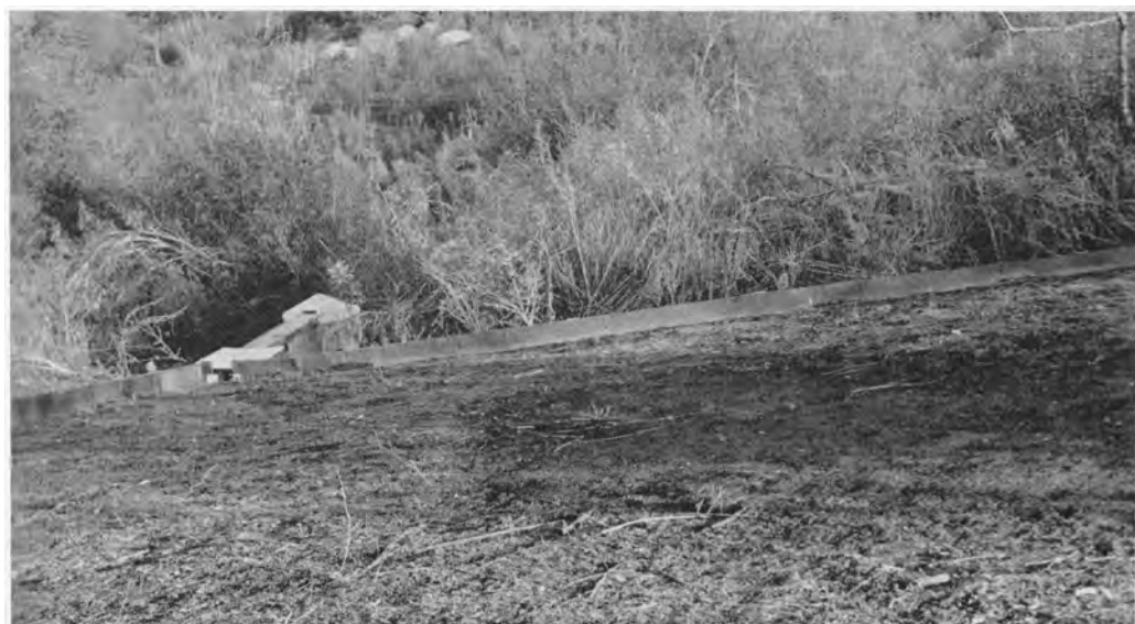
Illustrating the manner in which soil eroded from a denuded plot was caught and collected in a tank to be weighed at the end of the season.
