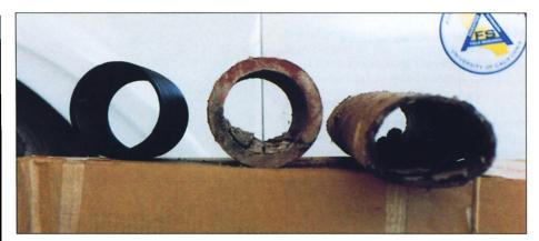
New plastic drain (left) compared with excavated clay and bituminous fiber drains installed in 1964.
