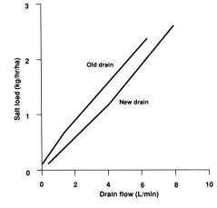
Fig. 2. Same drains show direct relationships between salt load and flow rate.
