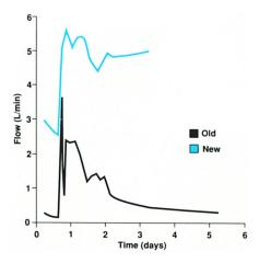
Fig. 1. Typical discharge hydrograph for old bituminous fiber and new plastic drains shows considerably higher flow rates in new drainlines after irrigation.
