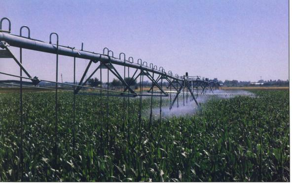
Experimental low-energy precise-application (LEPA) machine equipped with both spray nozzles (background) and drop tubes (foreground). "Bubblers" at the ends of the tubes discharge water directly into furrows (right). The system is credited in some areas with uniformities as high as 97 percent, but tests in California that considered machine movement patterns and soil intake rates showed lower uniformities.
