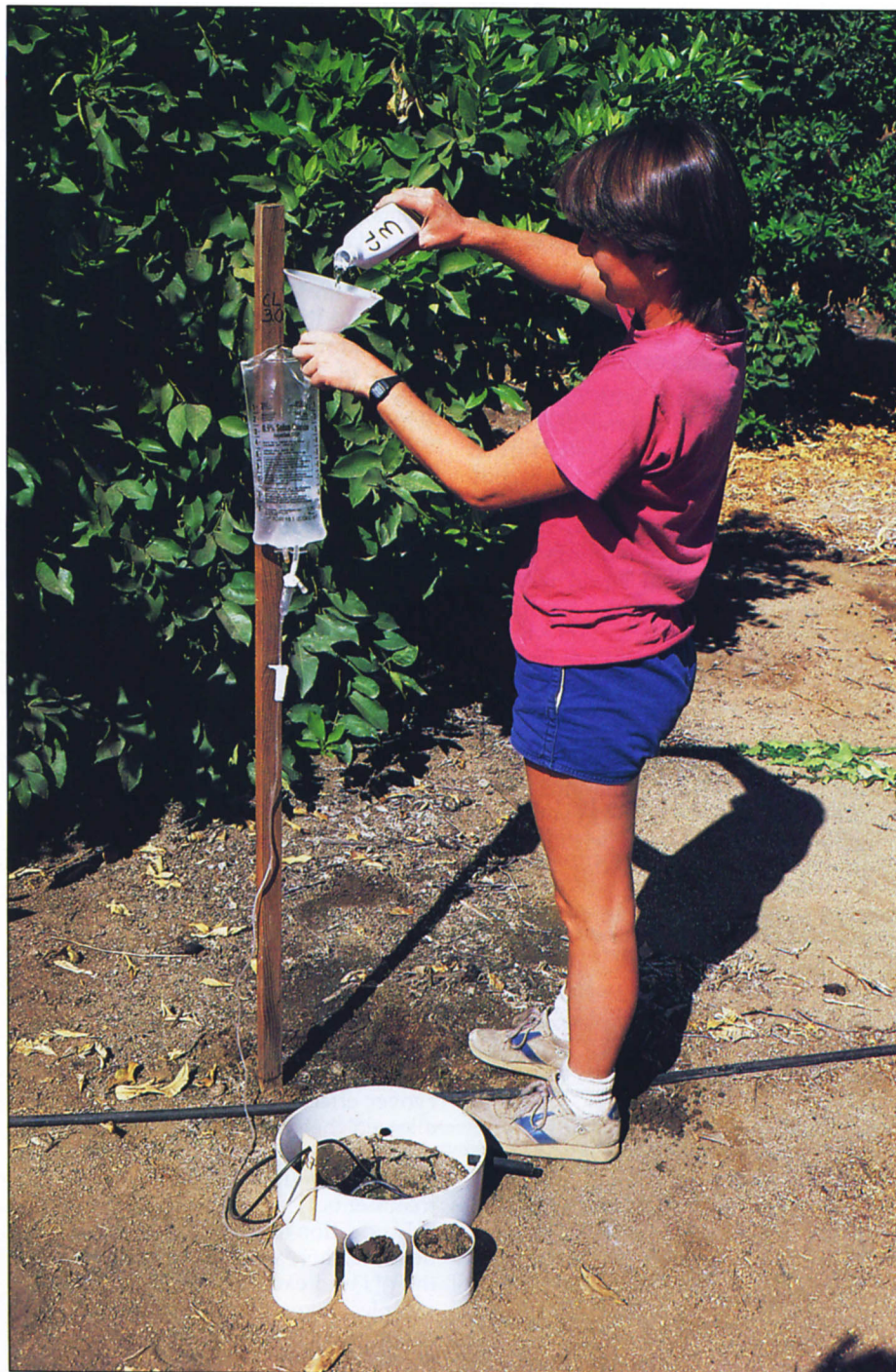
Ann Wildman adds a concentrated calcium salt solution to an intravenous bag, which feeds a measured amount of calcium to irrigation water flowing into the PVC infiltrator at bottom. Experiments showed that addition of calcium doubled or tripled the water infiltration rate over that of untreated low-salt water.
