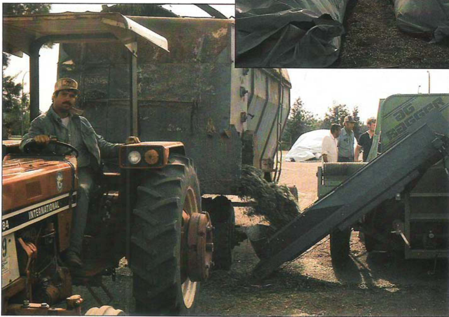
Growers run the chopped forage through a bagging machine (below), which ensiles the material in polyethylene silage bags (right).
