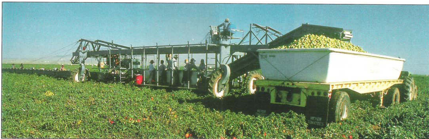
"Mechanical harvesting" doesn't say it all — a dozen or more laborers must work together to operate this tomato harvester, filling tractor trailers with green fruit destined to ripen fully on its way to market.
