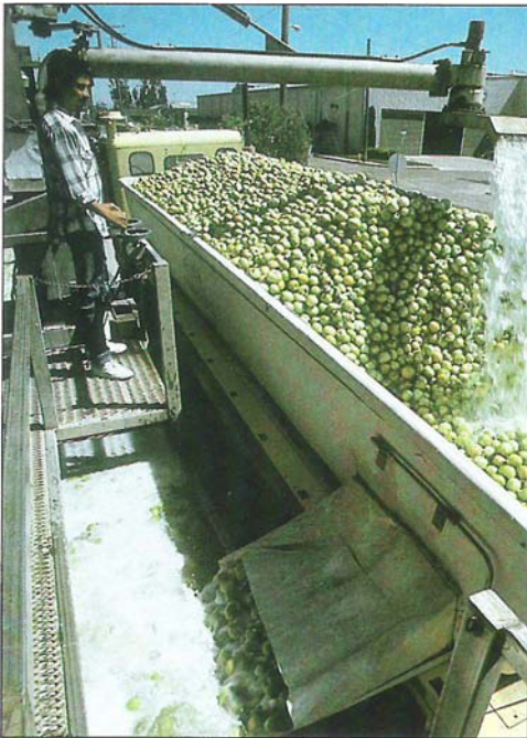
Trailer bins full of fresh-picked tomatoes ( left ) are flooded with water that will wash away pesticide residues and transport the fruit into the packing facility. After having been mechanically brushed, dipped, sprayed, and dried, fruit were sampled ( right ) at the end of the packing line.
