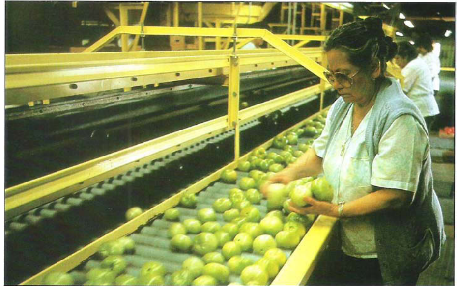
Trailer bins full of fresh-picked tomatoes ( left ) are flooded with water that will wash away pesticide residues and transport the fruit into the packing facility. After having been mechanically brushed, dipped, sprayed, and dried, fruit were sampled ( right ) at the end of the packing line.
