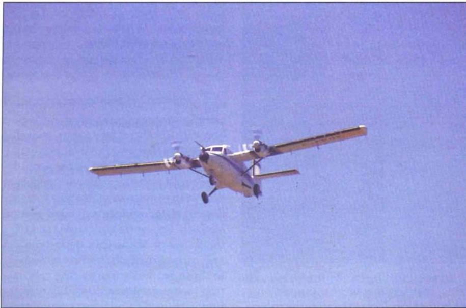
◀ A heavily instrumented Twin Otter research aircraft was used during the CODE experiment to measure ozone deposition to an irrigated vineyard in the San Joaquin Valley.
